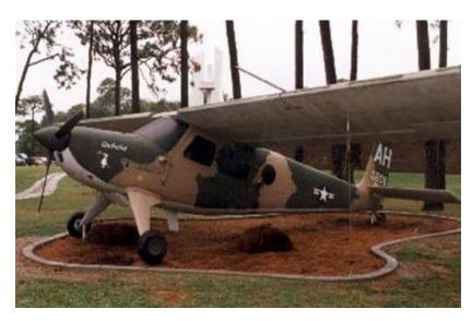
Primary Function: Courier, spotting and propoganda Builder: Helio Aircraft Corp. Power Plant: Single 295 hp. Textron Lycoming GO-480-G1D6 engine.
