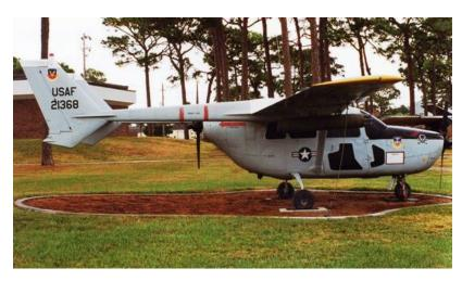
Primary Function: FAC Builder: Cessna Aircraft Corp. Power Plant: Two 210 hp. Continental 10-360C Engines Max Takeoff Weight: 4,900 lbs.
